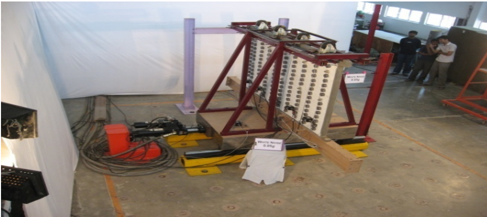
Figure 1: Uni-axial Shake Table
