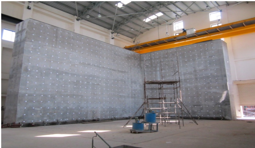
Figure 4: Pseudo-Dynamic Test Facility
